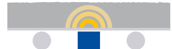
Schematic representation of neutron moisture measurement at a conveyer belt
